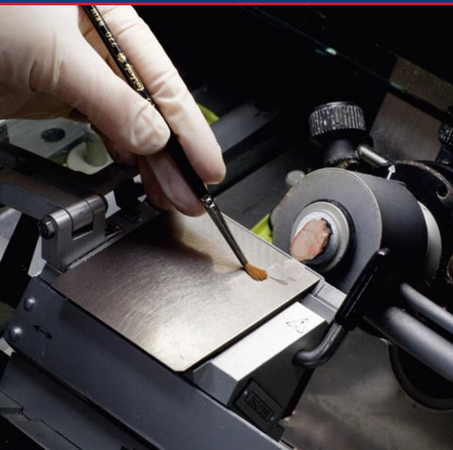
From frozen tissue 5µm sections are cut which can be used either for microscopy or for extraction of RNA and DNA.
